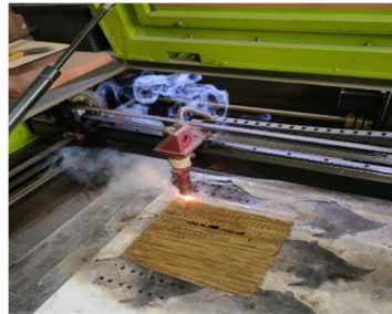
Figure 2.1(d): Laser cutting of the Composite
