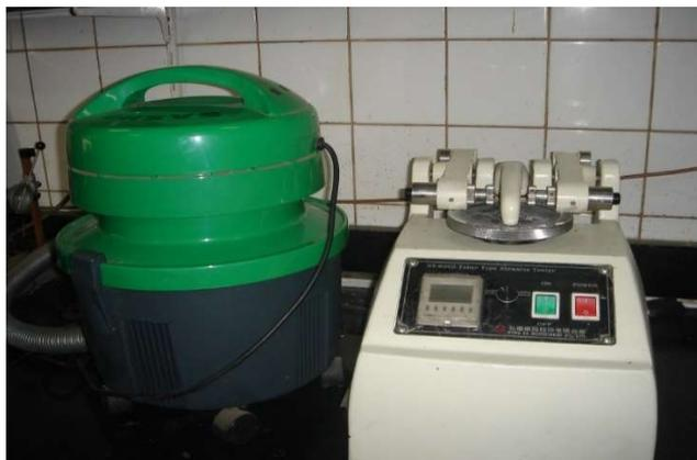
Figure 5. Abrasion tester, HT-8360, Japan
