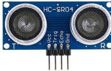
Figure 7. Ultrasonic Sensor [12].
