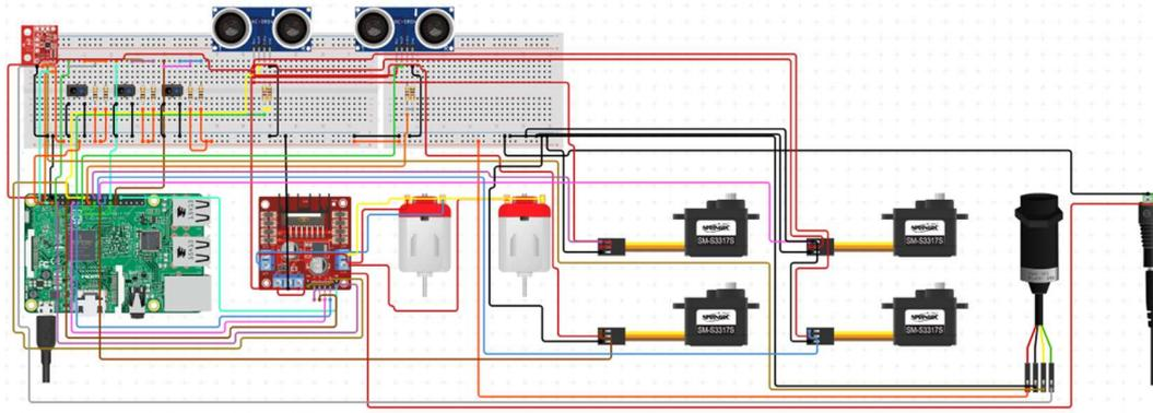
Figure 6. Schematic Diagram of Robocar
