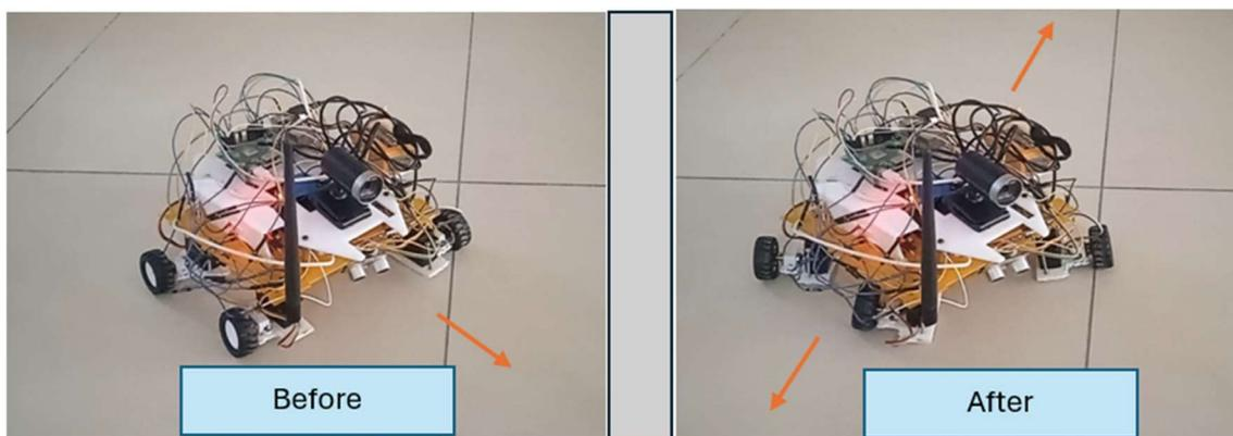
Figure 10. Demonstration of Diagonal Mode
