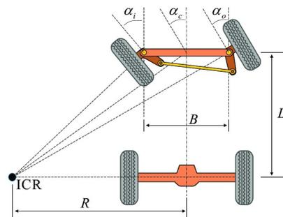
Figure 1. Illustration of a traditional two-wheel steering system [1].
