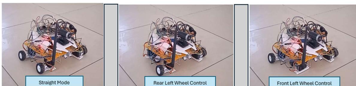
Figure 11. Demonstration of Independent Control Mode
