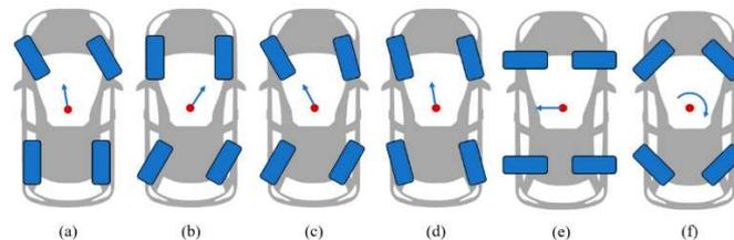
Figure 2. Illustration of a four-wheel independent steering system showcasing various maneuvers [2].
